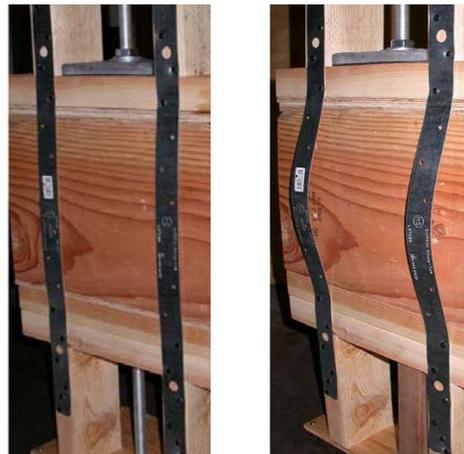
As the second photo shows, when the building shrinks the shrinkage compensator performs its intended function and tightens the rod. However, as the shrinkage compensator expands, the straps compress and the upper floor loosens
