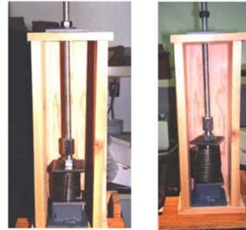
**Mixing Incompatible Systems** Straps and tie-down systems are often combined. The system to the left uses a shrinkage compensated tie-down system in combination with straps. At first glance this may look good but there are serious flaws.
