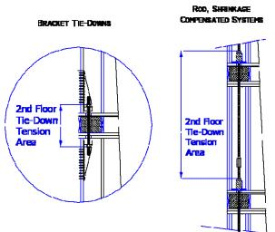
2. Select components for strength and fit compatibility. Designers select predesigned elements from look-up tables. Tables provide strength and deflection (elongation) at allowable load limits. The actual deflection is computed as a function of actual load.
